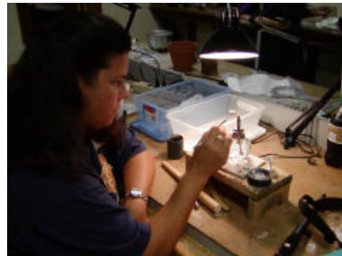
Classmate Debbie Dolphin works with wax to create a new design to be cast in metal.
