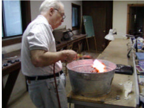
Fred shows the class how to use the centrifuge to inject silver into the mold.
