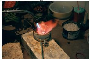
2. Light the torch and begin melting. You will know if you need casting flux, if you have some bright glowing floaties on top of the silver when it starts to ball up. If needed, remove torch and add casting flux (a pinch of Borax or a few grains of casting flux), and then reheat.
