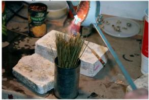
3. When it starts getting fluid (it will jiggle when you can shake it), lift crucible to the top of the broom straw. While keeping the
